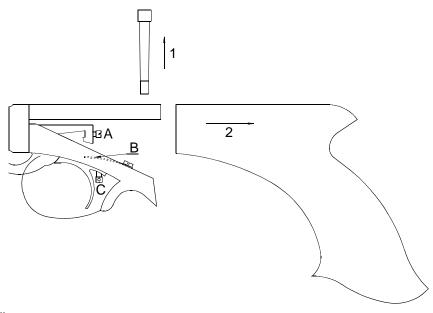
A = trigger adjustment screw
